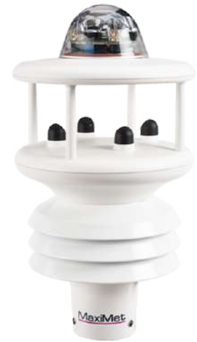
MaxiMet GMX600 measures 6 parameters including precipitation.
