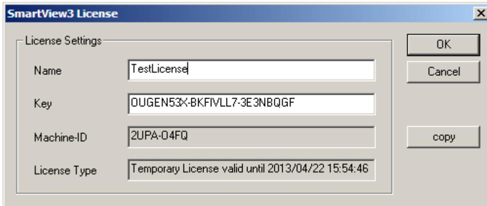
The license is bound to the PC hardware (identified by the specific Machine ID).
