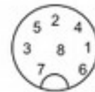
III 24: View on solder connection of the cable socket
