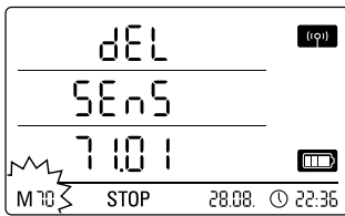
Example display: Log off function M70 selection for logging off the first selected sensor.
