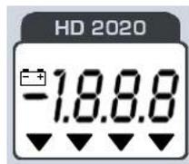
... an automatic test including battery power is performed and the instrument switches to standard mode.
