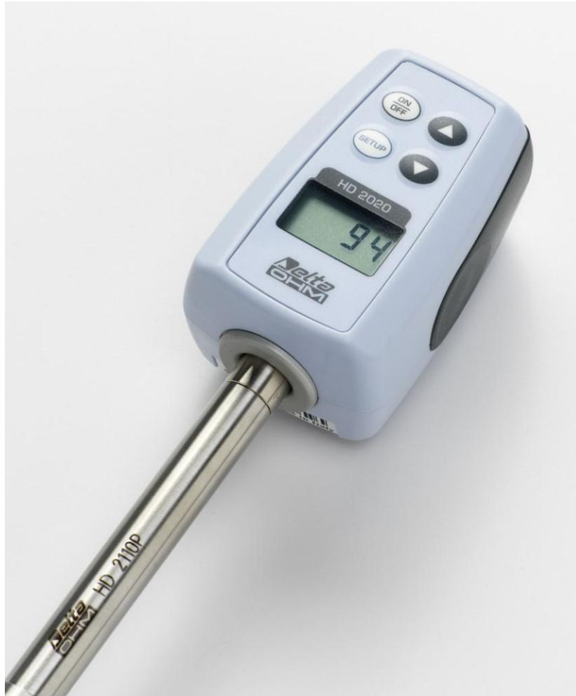
During calibration the HD2020 can be held in vertical position or placed on a flat surface. While measuring, you should move neither the microphone nor the calibrator; make sure that the worktable doesn't transmit vibrations. A small misalignment of the microphone and calibrator axes is allowed.
