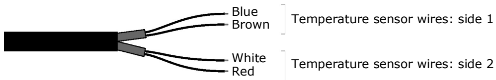
Fig. 6: Connection of probes TP32MTT.03.A and TP32MTT.03.C
